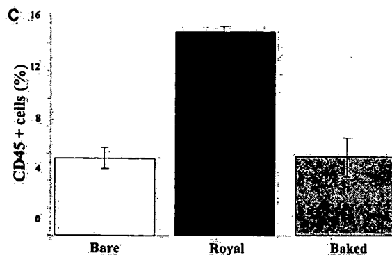
Figure 3. Photomicrographs (a; \times 200 ), extent of neointimal thickness (b; mm), and degree of inflammation (c; % porcine CD45-positive cells in neointima) 28 days after implantation of 9-mm stainless steel stents left intact (Bare; open bars), gold-coated NIR stents (Royal; solid bars), and flash-heated post-plated NIR stents (Baked; gray bars). Arrow indicates internal elastic lamina; *, sites of stent struts.
